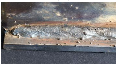
Fig 1. Spatter generated over welded surfaces
