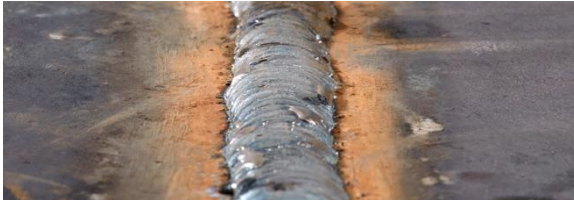
Fig 3. After use of anti-spatter liquid
