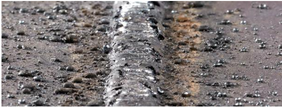
Fig. 2. Before use of anti-spatter liquid.
